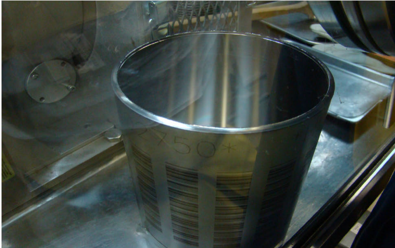
3013 Container Cut for Oxide Removal and Metallurgical Examination
